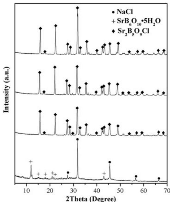
**Fig. 1** XRD patterns of the precursor (a) and the samples fabricated at different temperatures (b) 600 °C; (c) 700 °C; (d) 800 °C for 8 h.
