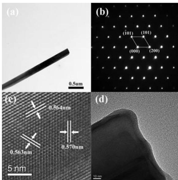
**Fig. 4** TEM image (a), SAED pattern (b), HRTEM image (c) and HRTEM image taken from the end tip (d) of the  $\text{Sr}_2\text{B}_5\text{O}_9\text{Cl}$  whisker fabricated at  $700^\circ\text{C}$  for 8 h.
