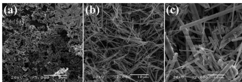
**Fig. 3** SEM images of the samples fabricated at different temperatures (a) 600 °C; (b) 700 °C; (c) 800 °C for 8 h.
