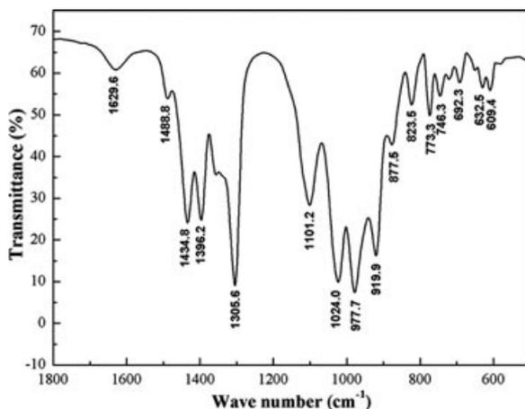
**Fig. 5** FT-IR spectrum of the  $\text{Sr}_2\text{B}_5\text{O}_9\text{Cl}$  whiskers fabricated at  $700^\circ\text{C}$  for 8 h.
