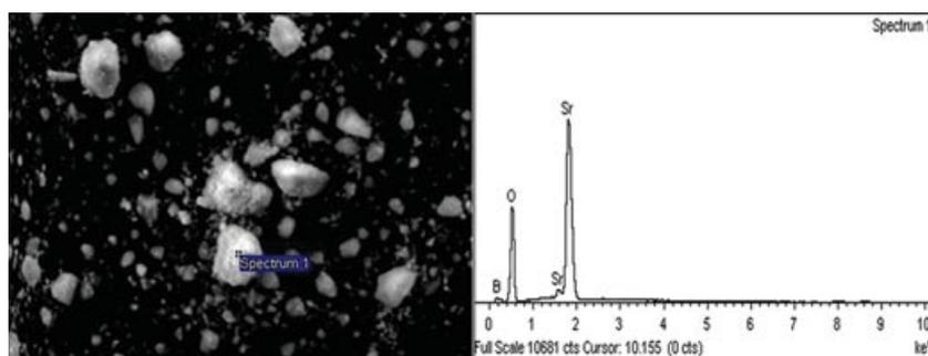
**Fig. 2** EDS spectrum of the final washed precursor.
